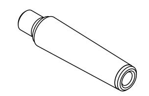
Use MT2 blank end arbor threaded for drawbar L/H end male thread M12
